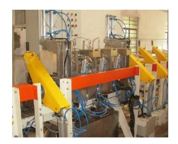
The Seamless Tube test systems is to test the defcets Longitudianally & Transverse oriented defects & Wall thickness measurement based on the International Standard in general E 213 or similar, etc. The Test Mechnism will have Immersion tank having various probes for the defects & wall thickness.
